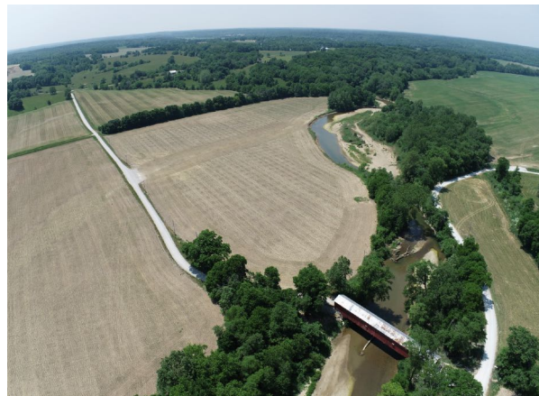
Drone photo flying high above Oakalla Covered Bridge, viewing a cutbank eroding into a cornfield. Channelized floodwaters that have swept gravel off the road re-enter the creek along the unvegetated cutbank, causing rapid bank retreat.
